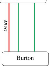
Current Configuration: 1-230 kV 1272 ACSR 2-115 kV 477 ACSR
