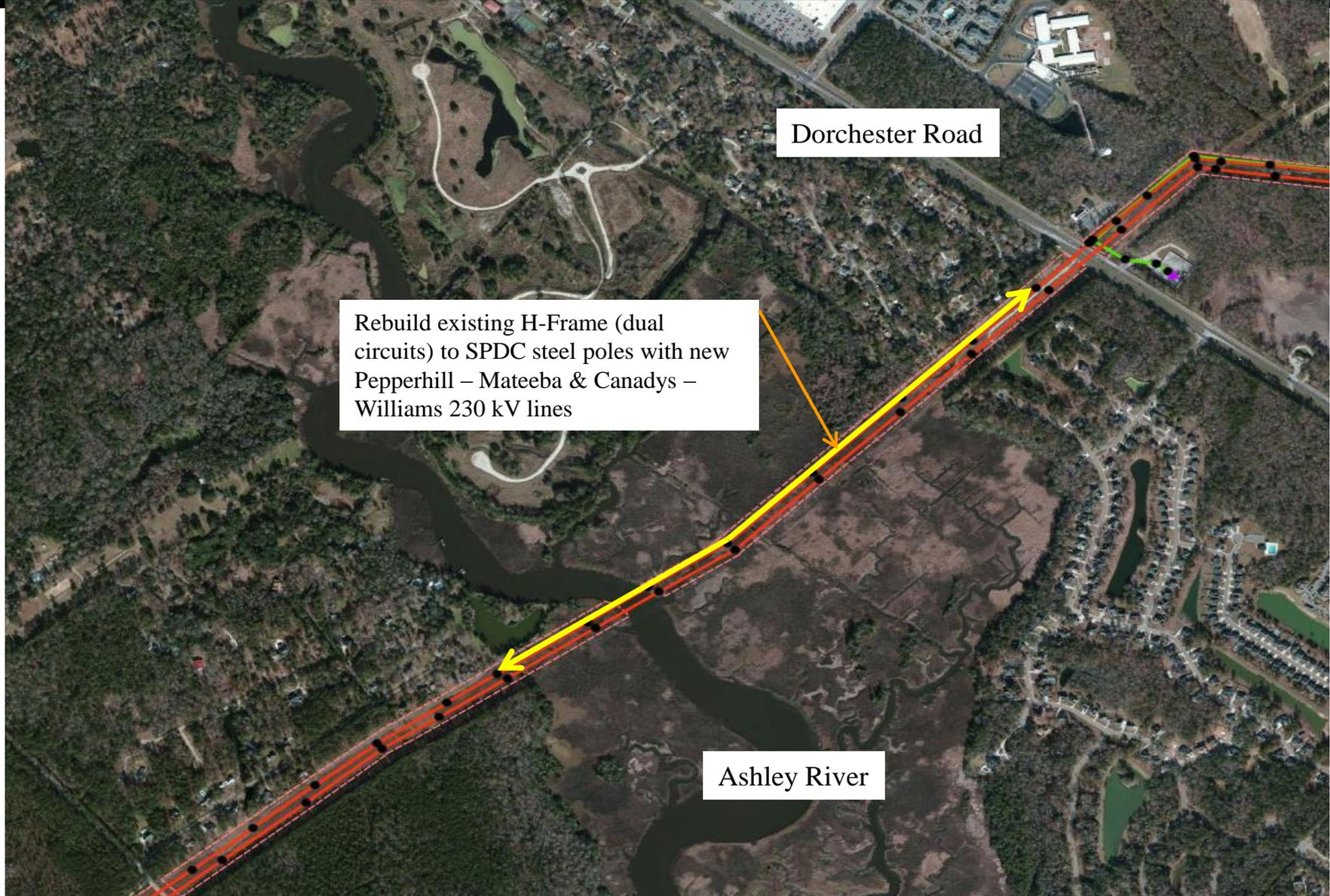
Rebuild existing H-Frame (dual circuits) to SPDC steel poles with new Pepperhill - Mateeba & Canadys - Williams 230 kV lines
